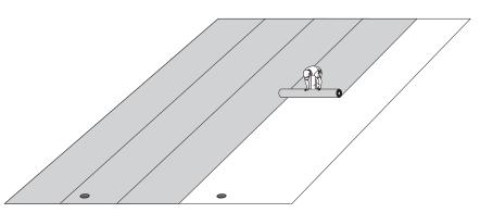
**Set Roof Drains:** Position Drain Boxes over the drains, adding sidewall elements as needed to match the system thickness.
