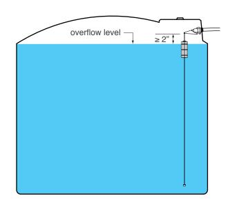
During wet period, rainwater fills the tank, the float ascends the cord, and the valve remains closed. To prevent backflow, the valve outlet must be 2"+ above the tank high water level.
