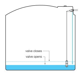
During dry periods, the water level drops until the float reaches the cord stop and opens the backup valve. The water rises a few inches, lifting the float and closing the valve.
